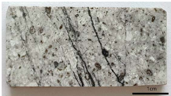
Image 1. TADD278, at 743.5 meters: Dacitic porphyry with intense sericitic alteration
