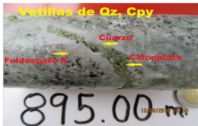
Figure 6 – Photographs E PORF 10 18 01. Showing porphyry-style copper and molybdenum mineralization.
