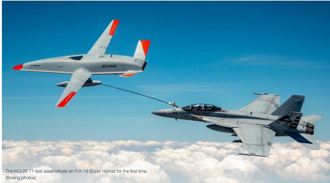
The MQ-25 T1 test asset refuels an F/A-18 Super Hornet for the first time. (Boeing photos)
