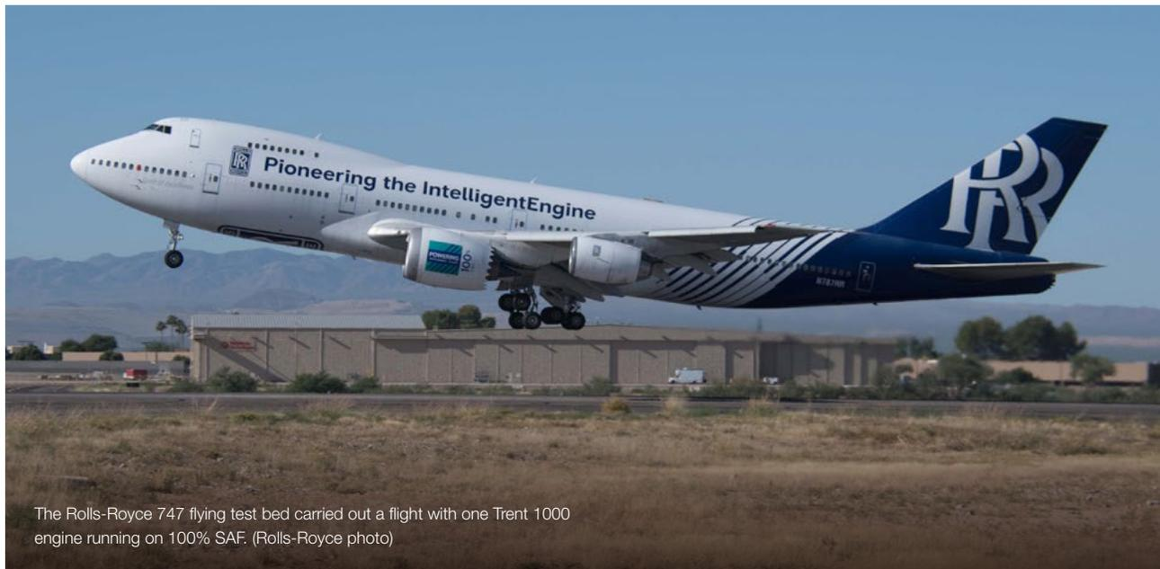
The Rolls-Royce 747 flying test bed carried out a flight with one Trent 1000 engine running on 100% SAF. (Rolls-Royce photo)
