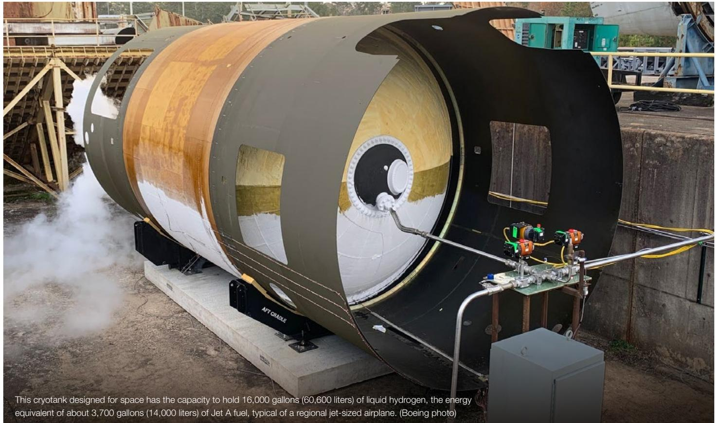
This cryotank designed for space has the capacity to hold 16,000 gallons (60,600 liters) of liquid hydrogen, the energy equivalent of about 3,700 gallons (14,000 liters) of Jet A fuel, typical of a regional jet-sized airplane. (Boeing photo)
